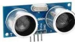
Gambar 4 Sensor Ultrasonik
