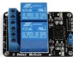
Gambar 3. Relay 220VAC/5 VDC [7]
