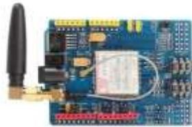
**Gambar 11.** Modul GSM SIM900
