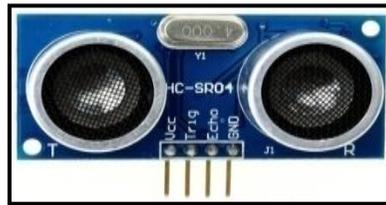
Gambar 7. Sensor *Ultrasonic* HC-SR04
