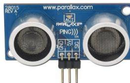
**Gambar 3.** Sensor Ultrasonik
